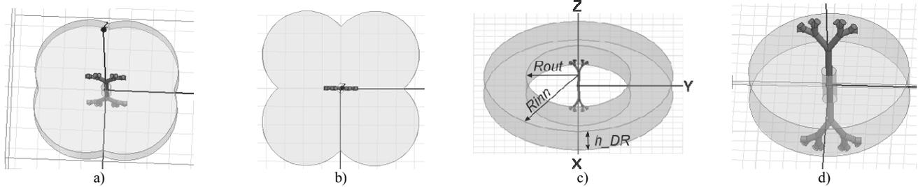
Fig. 4. Degenerate layout of the antenna: a) –  $X_{offset1} \div 4 = 6$  mm; b) –  $X_{offset1} \div 4 = 13$  mm; c) – at the confluence of the resonators in one ring; d) – minimizing the inner diameter of the ring resonator
