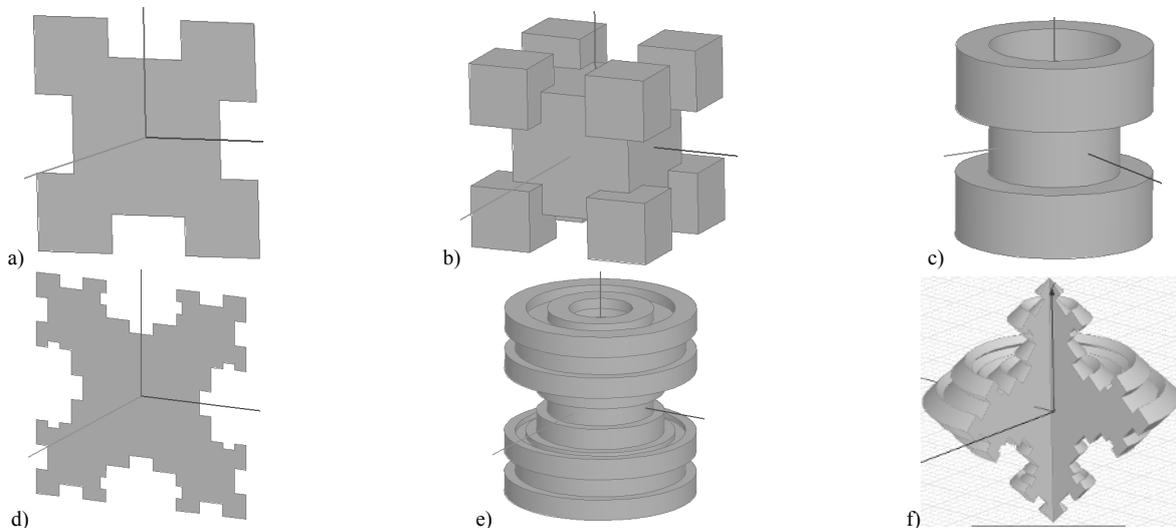
Fig. 11. Form of dielectric resonator structures based on Minkowski fractal ( $I=1, 2$ ) square frame: a) – template  $I=1$ ; b) – cubic shape for  $I=1$ ; c) – cylindrical shape for  $I=1$ ; d) – template  $I=2$ ; e) – cylindrical shape for  $I=2$ ; f) – partial cylindrical shape for  $I=2$  while rotating the pattern at a  $45^\circ$  angle in the plane  $YoZ$
